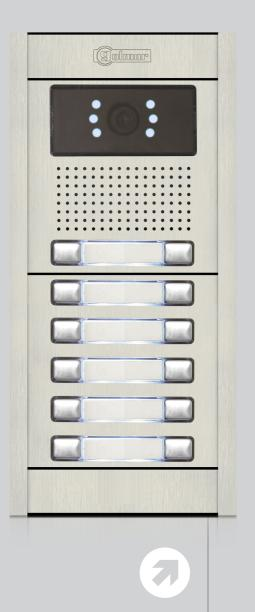
Front of 1.8mm. thick anodized extruded aluminium. Wall frame where electronic modules are to be inserted. Informative window manufactured in polycarbonate. Adjustable pan and tilt camera on video modules. Interchangeable single or double push buttons with stainless steel cover.
