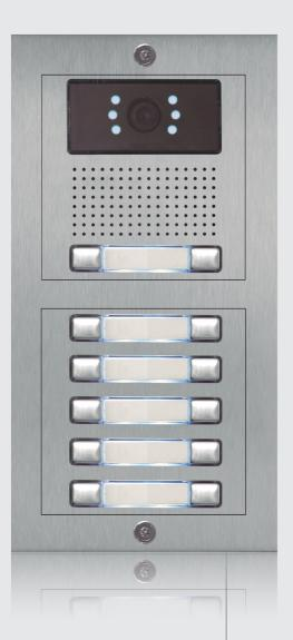
Front of 3mm. thick ANSI 316 stainless steel. Treatment to avoid fingerprint spots. Informative / camera window manufactured in polycarbonate. Adjustable pan and tilt color camera on video modules. Interchangeable single or double push buttons
