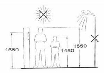
Drill one hole in the wall so that the upper part of the doorpanel is installed at a height of 1,65m.
