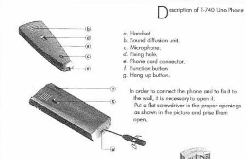
Do not install the device near heat sources, in places with dust or furnes. The phone can be fixed in a universal box or directly to the wall. To fix it directly to the wall, drill two 6mm holes in the position shown in the picture, by means of 6mm screws and  $\varnothing 3.5 \times 25mm$
