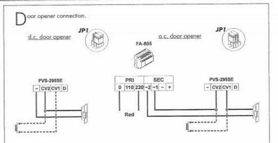
In order to open the door in any moment by means of an external button, connect the button between doorpanel terminals 'CV1' and 'CV2' as shown in the diagram.
